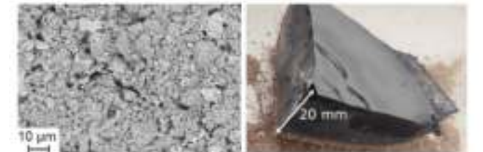
Scanning electron microscope image of the SMC-14 lunar regolith simulant (left) and a piece of the sintered and cracked material (right). Image: Aalen University, BAM/TU Clausthal
